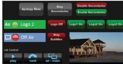
this level of device control within the automation client, the Smart Panel brings system management benefits by improving reporting and traceability, as commands made via the SmartPanel are incorporated into Marina Lite's AsRun log.
